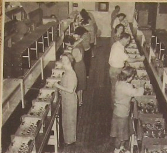
Partial view of the Hewlett-Packard assembly line in South Palo Alto. The testing equipment being assembled on the line at left is called "audio-oscillator," and on the right "harmonic wave analyzer."
